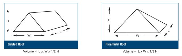
Recommended air changes in an attic are about 2-3 minutes per air charge (MIN/AC) to keep the temperatures down. (2 minutes in southern climates and 3 minutes in northern climates.)
