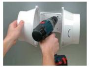
Fix the fan mounting plate on the flat surface.
