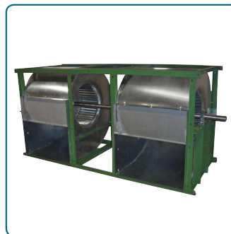
900 Series - Twin Double width, Double inlet, Framed heavy duty blower with pillow block bearing
