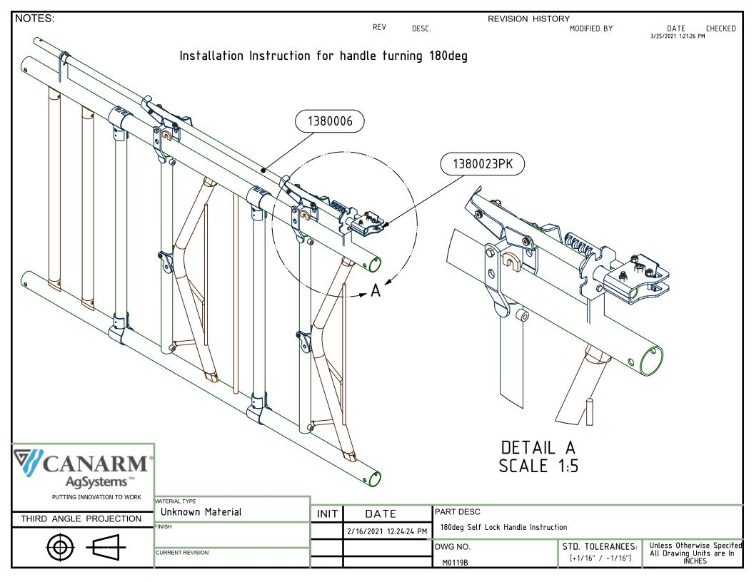
STEP 1: Redrill small existing hole in the turn rail with a 3/8" drill bit. Slide Mount Bracket onto the turn rail and attach Mount Bracket using the 1/4"x1" Hex Bolt and 1/4" Lock Nut
