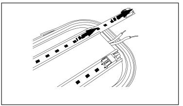
**4.** Connect the wire to the terminal block of LED strip,matching the "+" and "-" poles.
