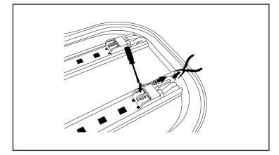
**3.** Replace a new LED strip to the aluminum plate, inserting follow the direction of the arrow.
