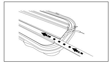
**2.** Pull out the LED strip from the aluminum plate the direction of arrow.
