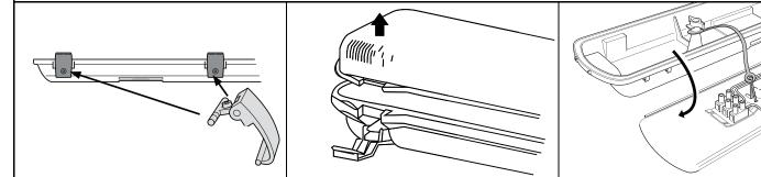
2. Screw two pieces metal bracket (packed in the accessory bag) to ceiling; install the housing to the metal bracket.
