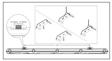
4. Screw two pieces metal bracket (packed in the accessory bag) to ceiling; install the housing to the metal bracket.
