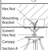
4. Feed wires and stem through the center hole of the mounting bracket. Slide a hex nut over the wires and start tightening onto the stem until "Section A" lines up with the arm assembly canopy (when the canopy is flush to the ceiling). Lock in position by tightening the (lower) hex nut against the mounting bracket.
