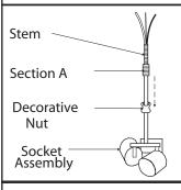
2。Unthread decorative nut from socket assembly and slide down the stem.
