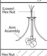
3。Slide arm assembly over socket assembly. Spin (lower) hex nut onto the stem approximately 1".
