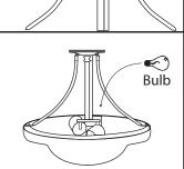
5. Attach the black wire from the light fixture to the black wire in the electrical box. Attach the white wire from the light fixture to the white wire in the electrical box. Connect the copper ground wire from the light fixture to the ground screw on the mounting bracket.
