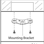
1. Assemble mounting bracket to electrical box using two electrical box screws (not included).
