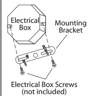
2. Mount the mounting bracket to electrical box using electrical box screws (not included). Make sure the studs on the mounting bracket are facing out from the electrical box.
