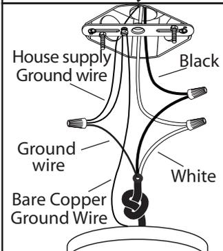
4. Firmly attach the fixture ground wire (bare copper) to the mounting bracket with the ground screw (by wrapping around the ground screw) and then connect it to the house supply ground wire with a wire nut. Connect black wire from fixture to black wire in electrical box and connect the white wire from fixture to white wire in electrical box.
