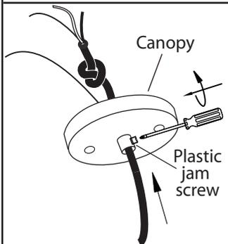
3. **Adjusting the length of flexible cord. Tighten the plastic jam screw after the length is set. For safety, do not release the knot inside canopy.**
