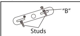
1. Loosen "B". Adjust stud to desired length and lock in place with "B".
