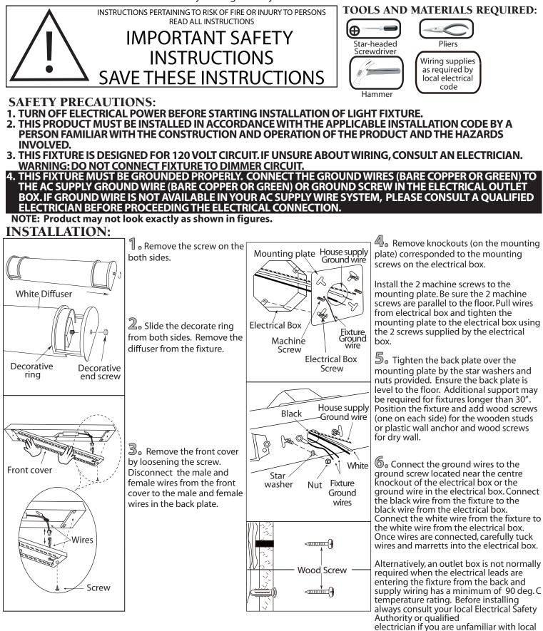
$\mathbb{Z}_{\circ}$  Reverse the process of Step 3, 2, 1 to install the fixture.
