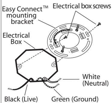
**2.** Attach Easy Connect™ mounting bracket to electrical box with electrical box screws (not included).
