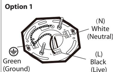
**3. Option 1:** Connect (push) electrical wires from electric box (house wiring) into correct inserts.
