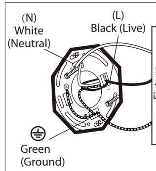
**4.** Connect (push) electrical wires from fixture into correct inserts.
