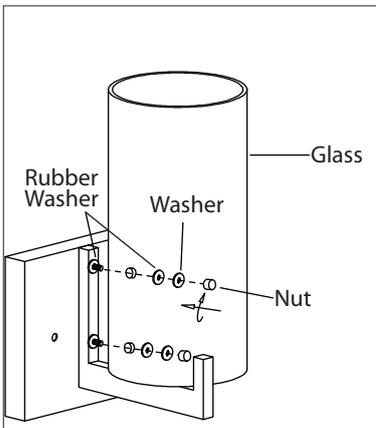
**1.** Secure the glass to the fixture with the rubber washers, washers and nuts.
