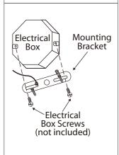
Mount the mounting bracket to electrical box using electrical box screws (not included). Make sure the studs on the mounting bracket are facing out from the electrical box.
