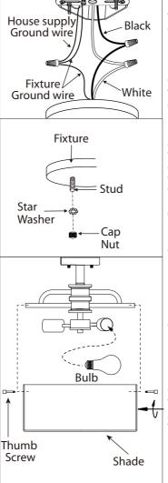
Connect the ground wires (bare copper or green) from your fixture to the ground wire (bare copper or green) or ground screw in the electrical box. Connect the black wire from the fixture to the black wire in the electrical box and connect the white wire from the fixture to the white wire in the electrical box.
