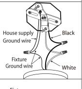
2 Connect the ground wires (bare copper or green) from your fixture to the ground wires (bare copper or green) or ground screw in the electrical box. Connect black wire from fixture to black wire in outlet box and connect the white wire from fixture to white wire in electrical box.
