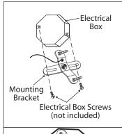
$\mathbb{1}_{\circ}$  Mount the mounting bracket to electrical box using electrical box screws (not included). Make sure the studs on the mounting bracket are facing out from the electrical box.
