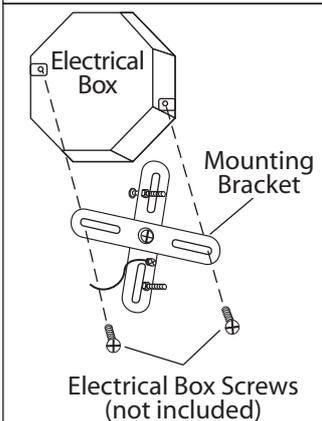
3. Mount the mounting bracket to electrical box using electrical box screws (not included). Make sure the studs on the mounting bracket are facing out from the electrical box.
