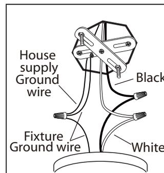
4. Connect the ground wires (bare copper or green) from your fixture to the ground wire (bare copper or green) or ground screw in the electrical box. Connect the black wire from the fixture to the black wire in the electrical box and connect the white wire from the fixture to the white wire in the electrical box.
