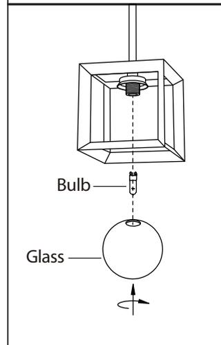
7. Install proper bulb type and wattage (not included). (FROST bulb gives better effect on the glass.)
