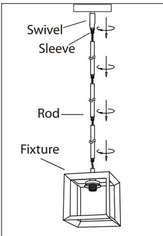
1. Install the length of rod that is required by threading wire through the rod and screwing it to the fixture. Install swivel to the rod, ensuring that the sleeve is at the swivel.
