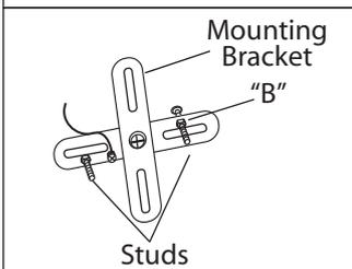
2. Loosen "B". Adjust stud to desired length and lock in place with "B".
