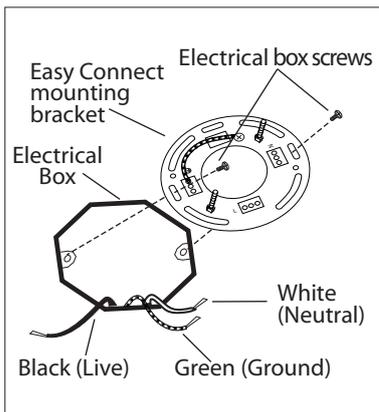
**1.** Attach easy connect mounting bracket to electrical box with electrical box screws (not included).
