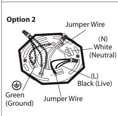
**Option 2:** For multiple green (ground), black (live) and white (neutral) wires joined in the electrical box (house wiring), attach a single "green", "black" and "white" jumper wire before connecting. Strip 7mm from the 6" jumper wires (AWG 12-24) supplied. Then connect (push) wires into the correct inserts.
