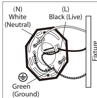
**3.** Connect (push) electrical wires from fixture into correct inserts.
