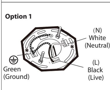
**2. Option 1:** Connect (push) electrical wires from electric box (house wiring) into correct inserts.
