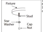
Tuck electrical wires into outlet box and position fixture over studs on mounting bracket assembly. Secure fixture in place with star washer(s) and cap nut(s).
