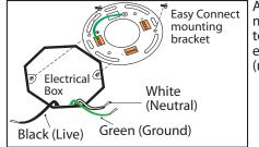
Attach easy connect mounting bracket to electrical box with electrical box screws (not included).
