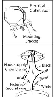
$1_{\circ}$  Attach mounting bracket to electrical outlet box with electrical box screws (not included).
