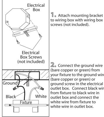
your fixture to the ground wire outlet box. Connect black wire
