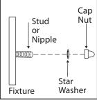
Tuck electrical wires into outlet box and position fixture over studs or nipple on mounting bracket assembly. Secure fixture in place with star washer(s) and cap nut(s). Note: If required, assemble body and spread the arms of the fixture out evenly.
