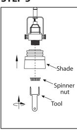
Remove spinner nut from socket. Position shade on lamp and secure with spinner nut.
