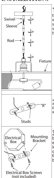
lostall the length of rod that is required by threading wire through the rod and screwing it to the fixture. Install swivel to the rod, ensuring that the sleeve is at the swivel.
