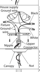
$\circ$  Once connections of wires are completed, carefully tuck wires and wire nuts into the outlet box making sure no bare wire (on the black and white) is visible at the wire nuts. Slide canopy into position and tighten in place by nut into position.
