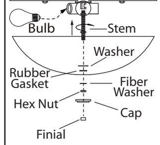
10. Install specified bulb type and wattage (not included).
