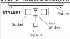
Align the center hole in the fixture with the nipple in the mounting bracket. Secure the fixture in place with a cap nut.
