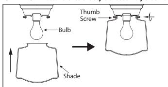
Install specified bulb type and wattage (not included).
