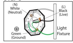
Connect (push) electrical wires from fixture into correct inserts.
