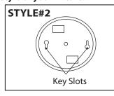
Tuck the electrical wires into the electrical box and position the "key slots" over the support screws. Turn and lock the support screws into the "key slots". Tighten the support screws into place.
