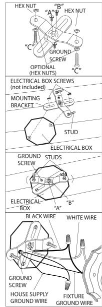
□ o Assemble the mounting bracket(2 pieces) as per drawing."A" and "B" screws should only be snug at this point. Screw "C" may be tightened and locked in place with hex nut(s)(if mounting bracket holes are untapped, an additional two hex nuts are required). The ground screw should then be attached to the mounting bracket (do not tighten).
