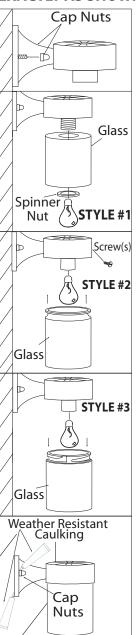
5. Once connections of wires are completed, carefully tuck wires and wire nuts into the outlet box making sure no bare wire (on the black and white) is visible at the wire nuts. Install the light fixture to the wall by aligning the hole(s) in the fixture with the studs or nipple on the mounting bracket. Secure in place with cap nut(s) and star washer (s).
