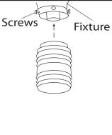
5. Position glass over the bulb and fasten in place with the jam screw.
