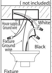
2. Firmly attach the fixture ground wire (bare copper) to the mounting bracket with the ground screw (by wrapping around the ground screw) and then connect it to the house supply ground wire with a wire nut. Connect the black wire (or wire with marking) from the fixture to the black wire in the electrical box and connect the white wire from the fixture to the white wire in the electrical box.
