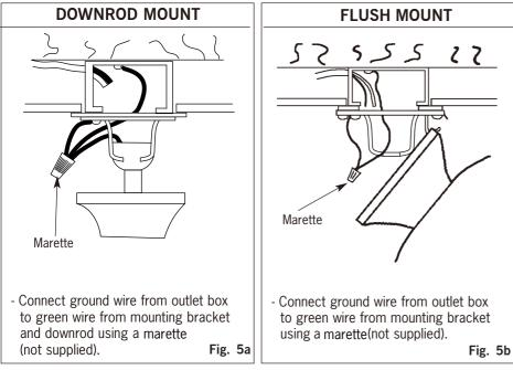
**NOTE**: Once ground wires are connected, carefully tuck wires and marette into the outlet box making sure that the wires are clear of the hemisphere and downrod when positioned in mounting bracket (Downrod Mount Only).
