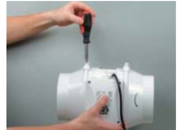
Secure latches by screws.
