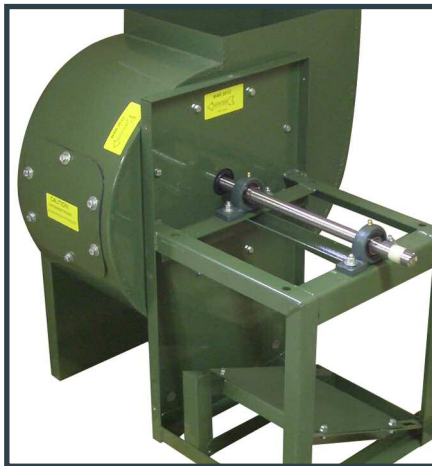
MOTOR AND DRIVE COMPARTMENT WITH COVER REMOVED TO ILLUSTRATE 3 SIDE MOTOR ACCESS AND SLOPED MOTOR BASE FOR BELT TENSIONING.
