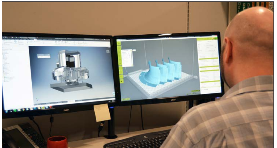
Tim Hull, Senior Design Engineering Technician at CANARM uses solid modelling software to design an A2X Spun Aluminum Exhauster. He also uses 3D printing technology to allow for multiple rapid design iteration and low cost prototyping, prior to expensive tool ups.
