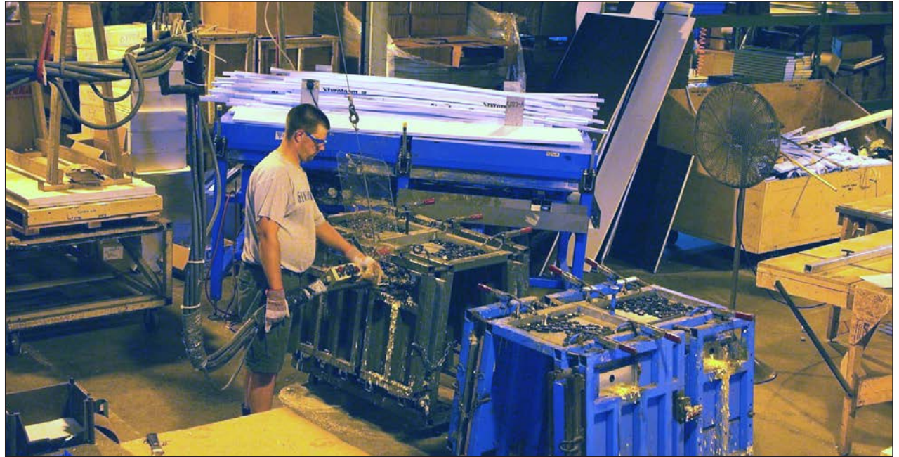
Chris Eckford injects foam into heated livestock waterer parts.
