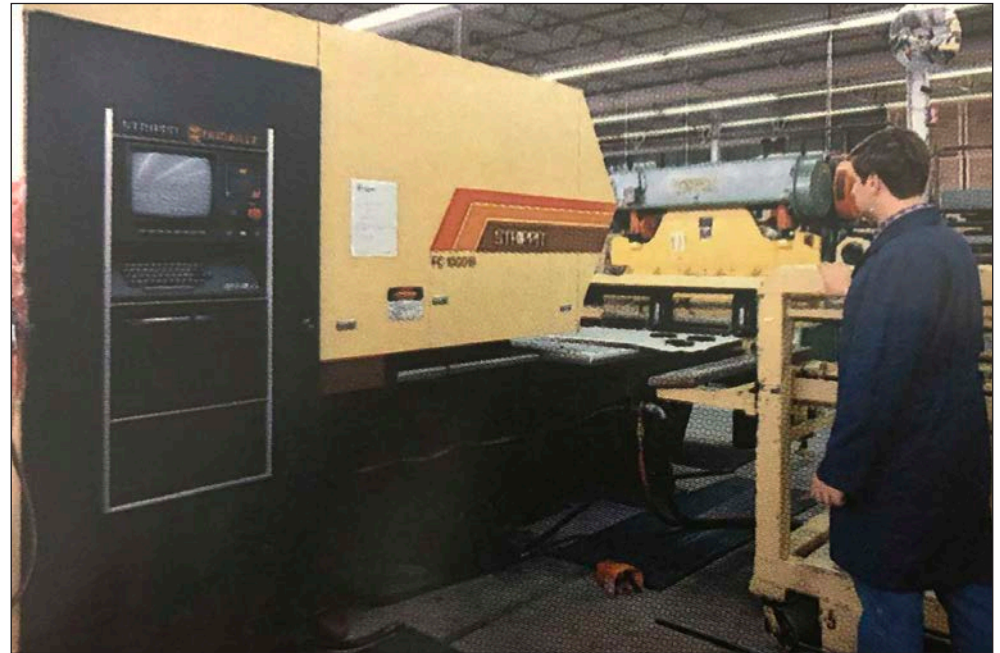
Computer-controlled turrett punching centre with automatic load and unload.
