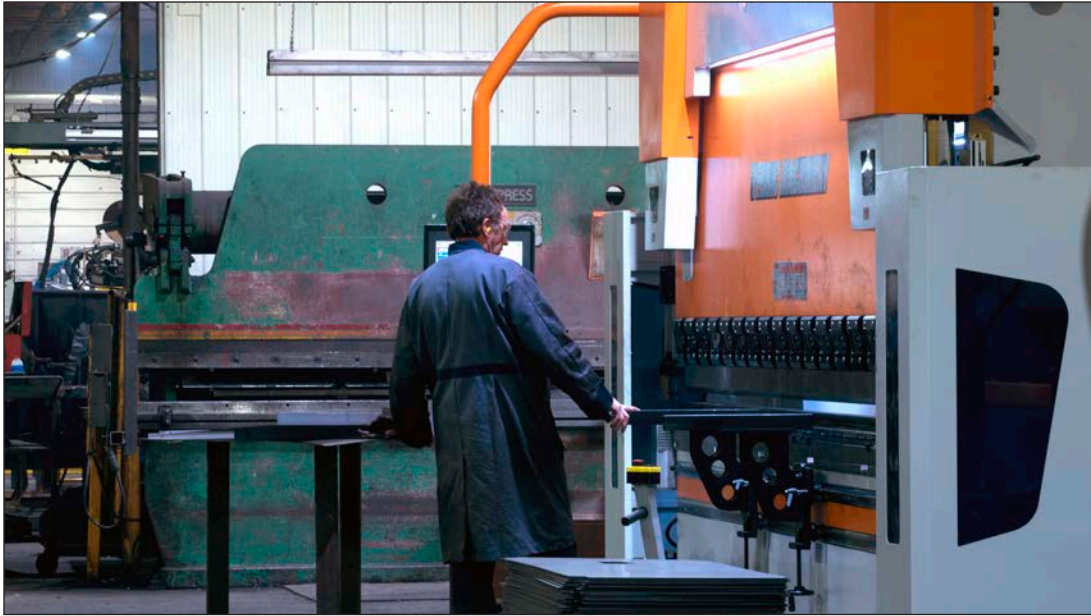
Louis Drost, Metal Fabrication Lead Hand. Louis has been at the Arthur location since March 1986. He is seen here making heated waterer parts on the ERMAKSAN 193 U.S. TON CNC BRAKE PRESS. (new in 2017)
