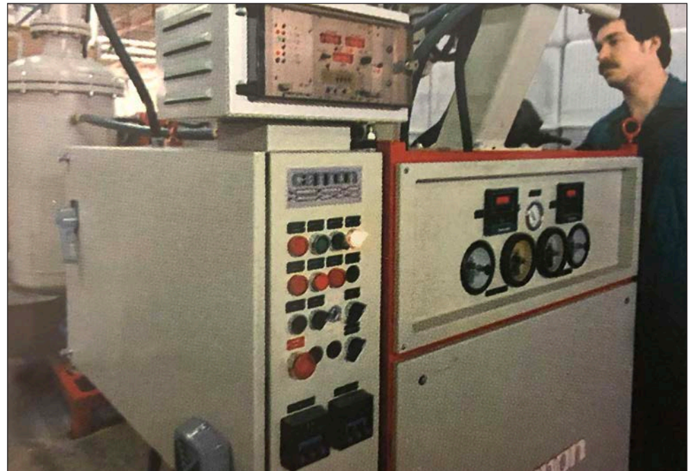
Computer-controlled foam injection.
